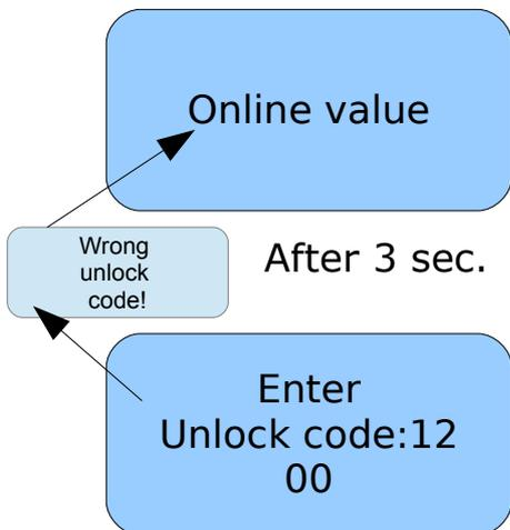
1. At first keep the enter key (  $\frac{\Delta}{\Sigma}$  ) pressed for three seconds. Than the S 201 will ask to enter the unlock key.
