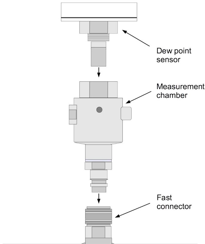
1. connect the sensor with the measurement chamber.
