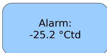
By pressing the Enter key the current alarm threshold value can be shown and it will go back to online value automatically in 3 seconds.
